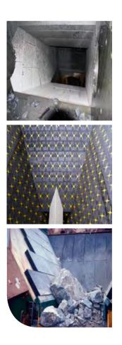
**Trellex Poly-Cer** The hard ceramic surfaces provide unsurpassable wear resistance while the elasticity of the rubber absorbs the impact of blows. Poly-Cer is used in many quarry and mining applications, particularly where abrasion is high and the angle of impact of material against the plates is small.
