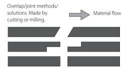
For cutting joint/s as shown we recommend to use same tooling intended for wood.
