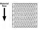
Ceramic inserts should be placed in a zigzag pattern against the material flow, as shown above.
