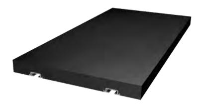
Excellent wear resistance in applications with both impact and sliding wear. The vulcanized aluminum profiles allow for fewer fixing points than steel-reinforced wear plates. Trellex PT wear plates reduce noise and vibrations, and are lighter compared to conventional steel lining.
