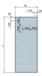
Calculate with 20 fixings/m<sup>2</sup>.
