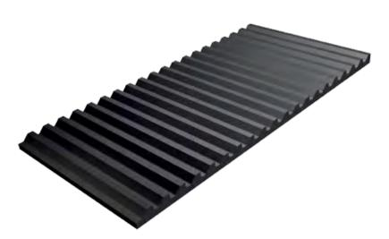
Excellent wear resistance in applications with both impact and sliding wear. The steel backing guarantees secure fixing so that the wear plates remain together even if the lining is exposed to extremely abrasive and sharp particles. The serrated surface has been designed to provide optimal life for material with impact angles between 15° and 50°. Trellex SP wear plates reduce noise and vibrations, and are lighter compared to conventional steel lining.
