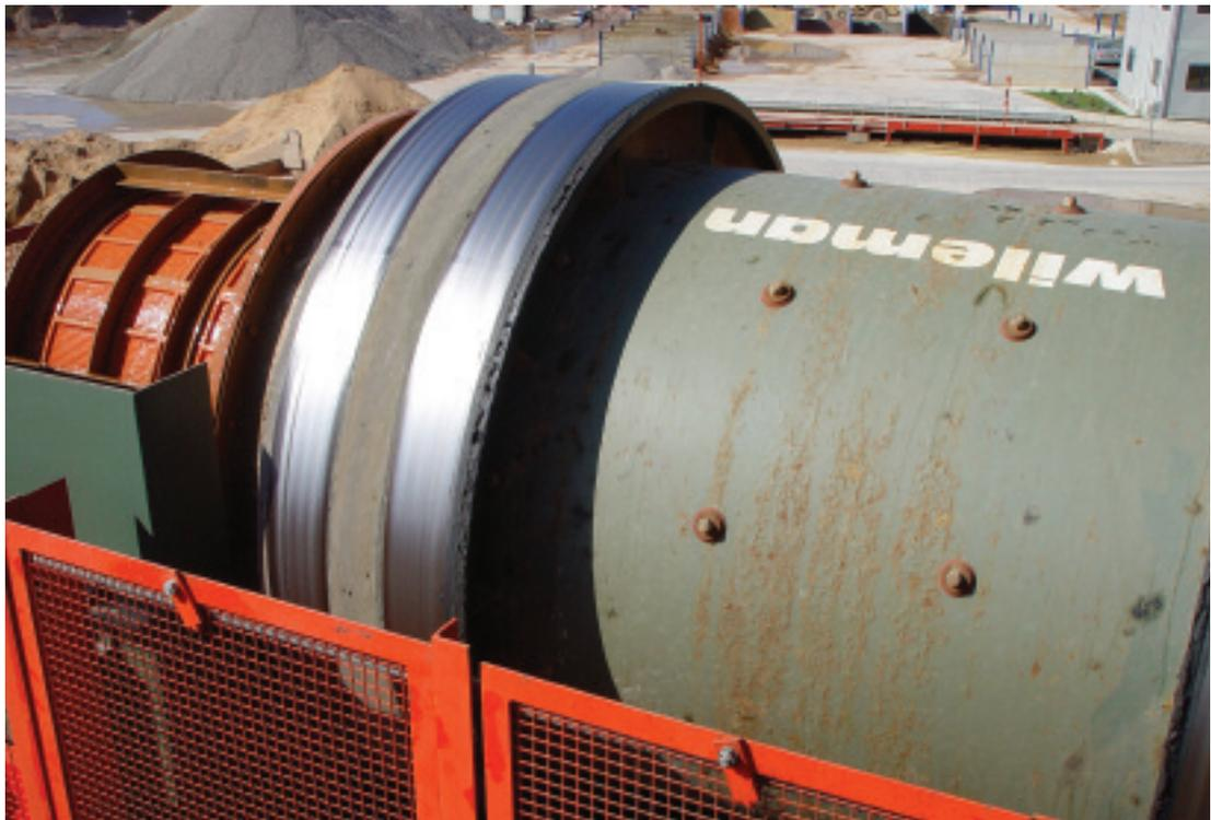
material passes over the trommel for further processing.
