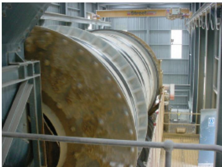
Wileman scrubber barrels are robust and include roller paths that ensure a concentric and smooth drive
