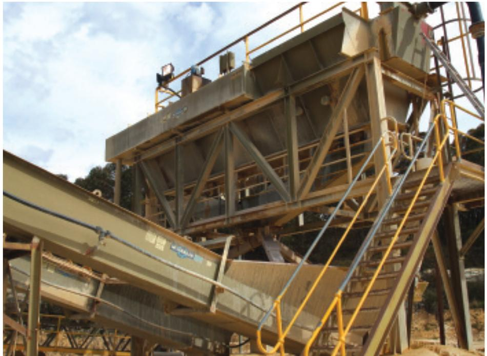
A typical classifying tank in operation
