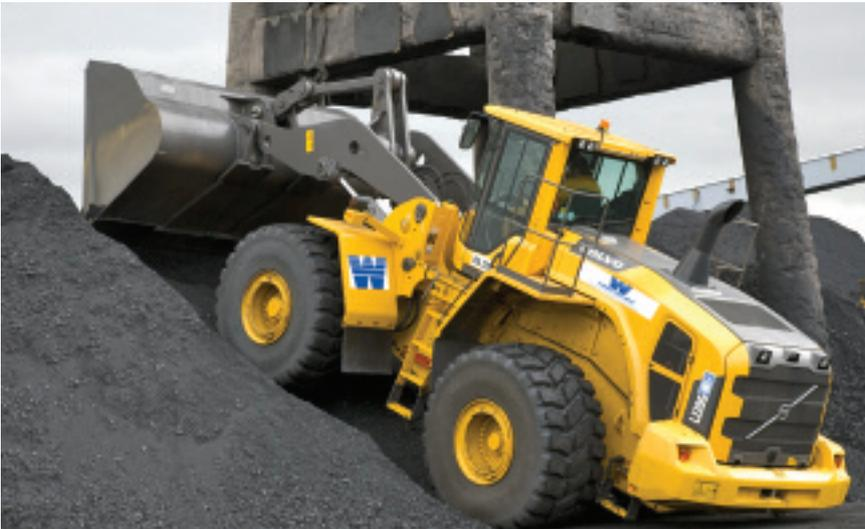
The Volvo L220G wheel loader is powered by a Tier 4 Interim engine with cooled EGR technology
