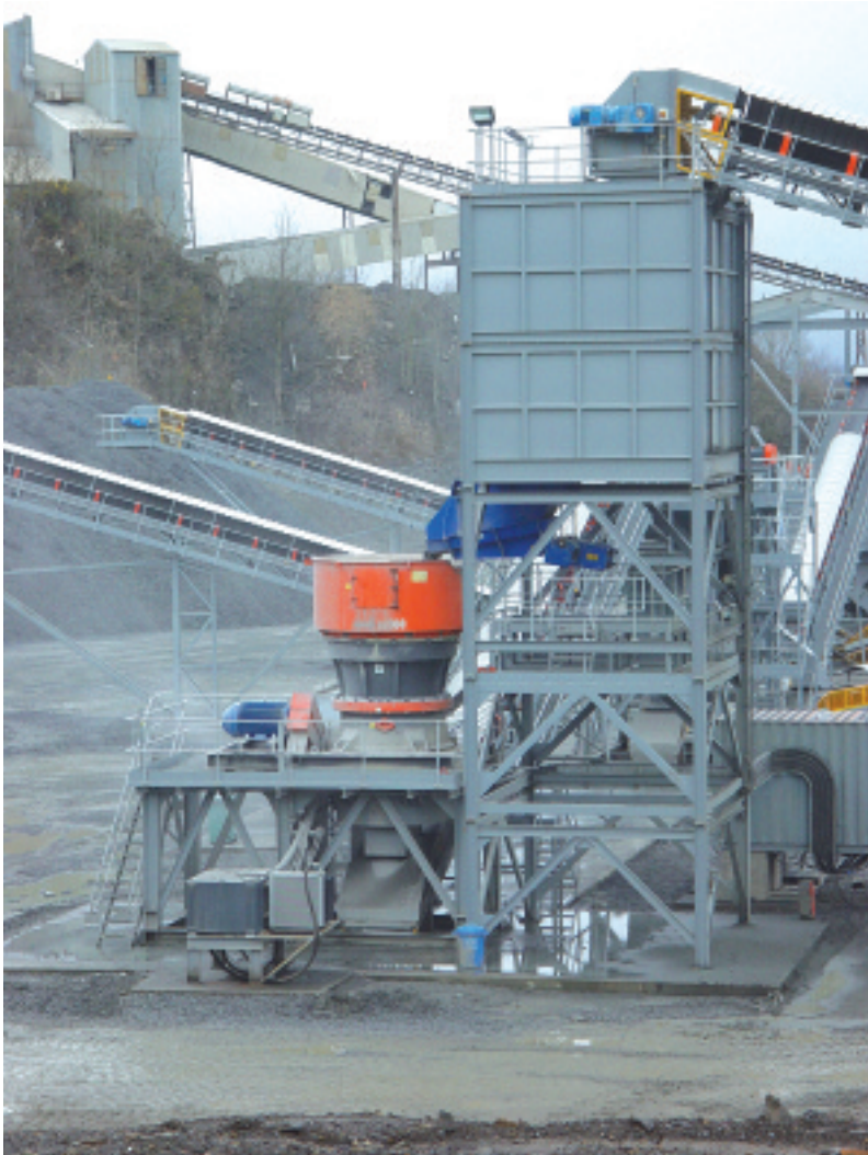
The new Sandvik CS660 secondary cone crusher and 100-tonne line capacity feed hopper mounted on a modular stacking frame
