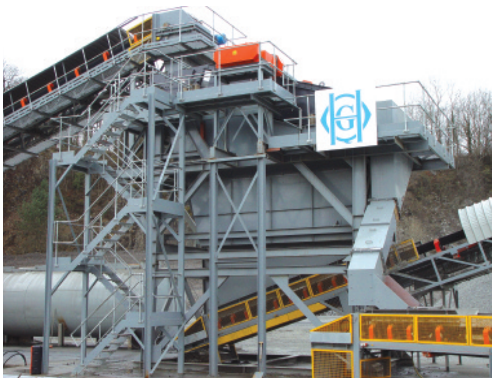
The new Sandvik MSO 2460S single-deck screen which takes out -40mm Type 1
