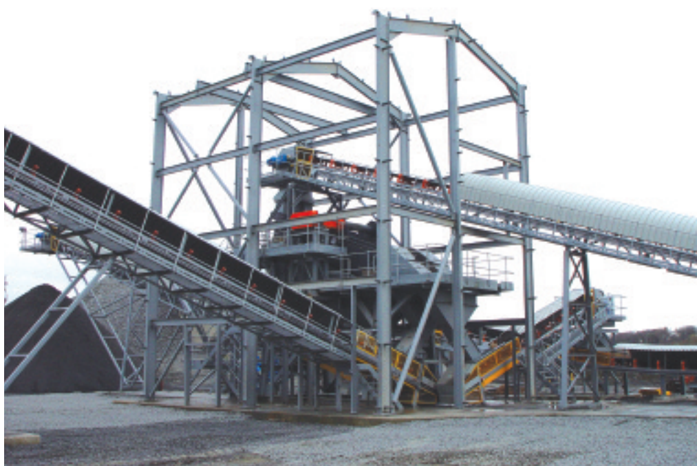
The new Sandvik MSO 2460D double-deck screen which produces -20mm +5mm and 0-5 dust
