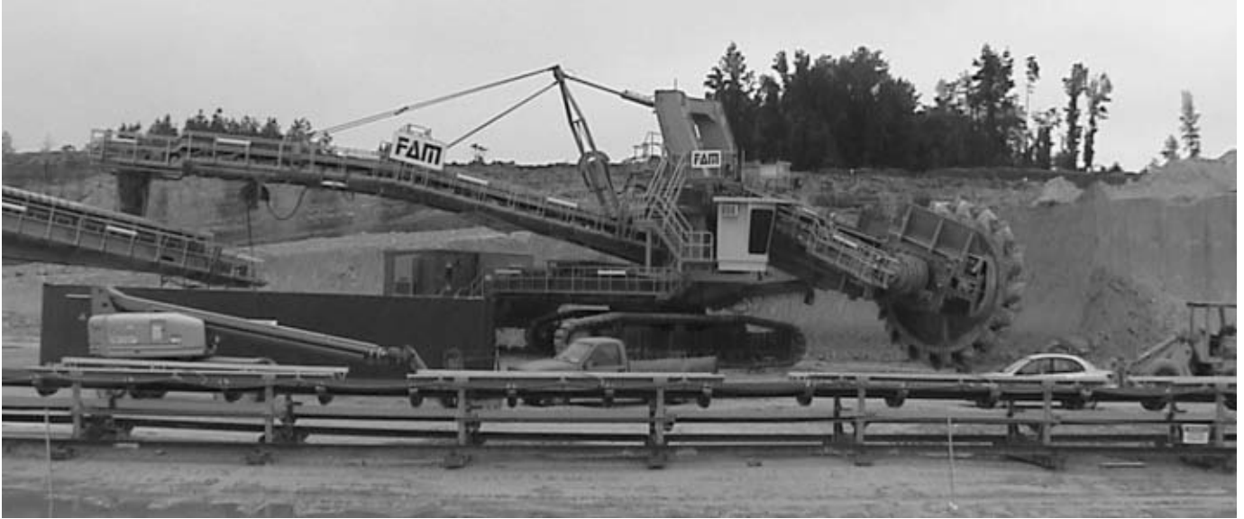
Excavator in a US cement application. Two Motorized Pulleys type 800H drive both the incoming & outgoing conveyors.
