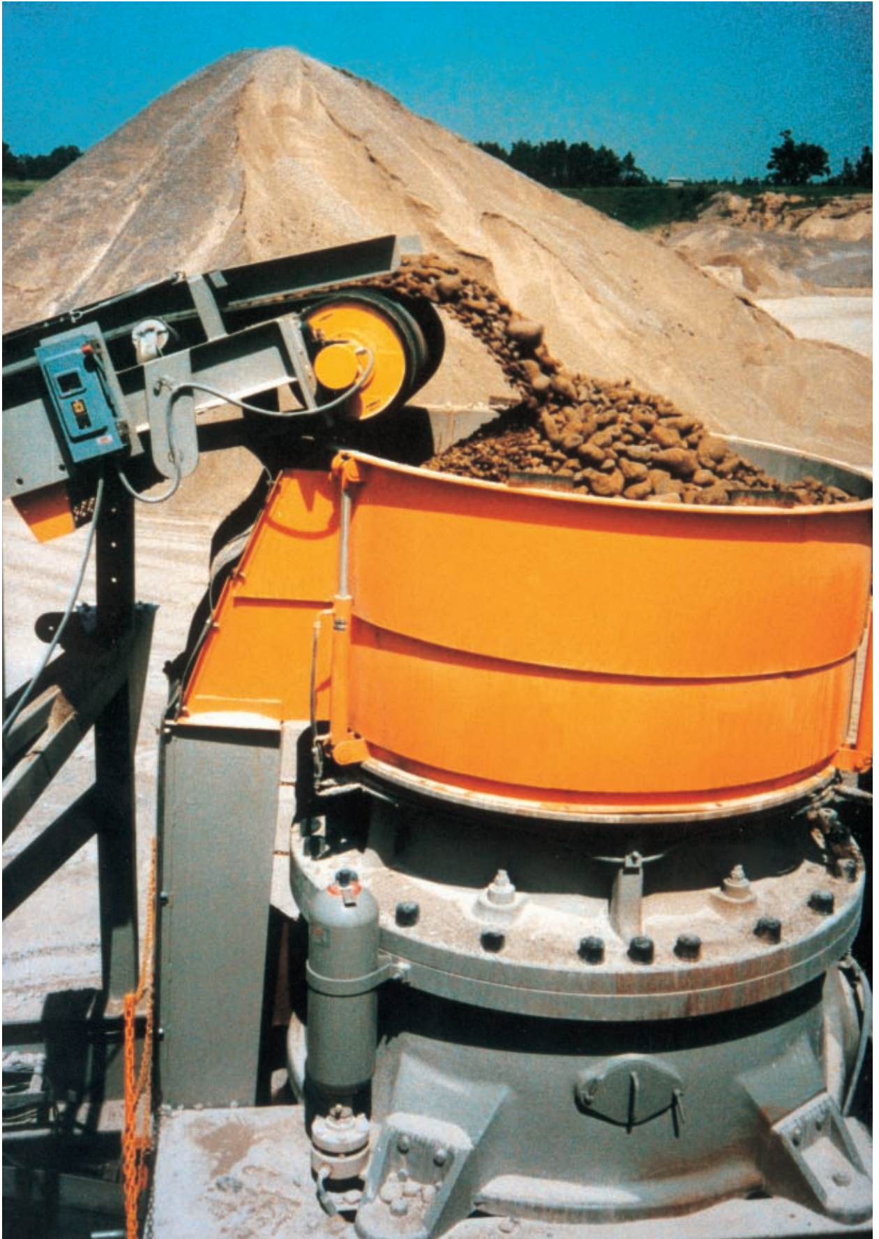
Crushing & Screening – A motorized pulley in its right element!
