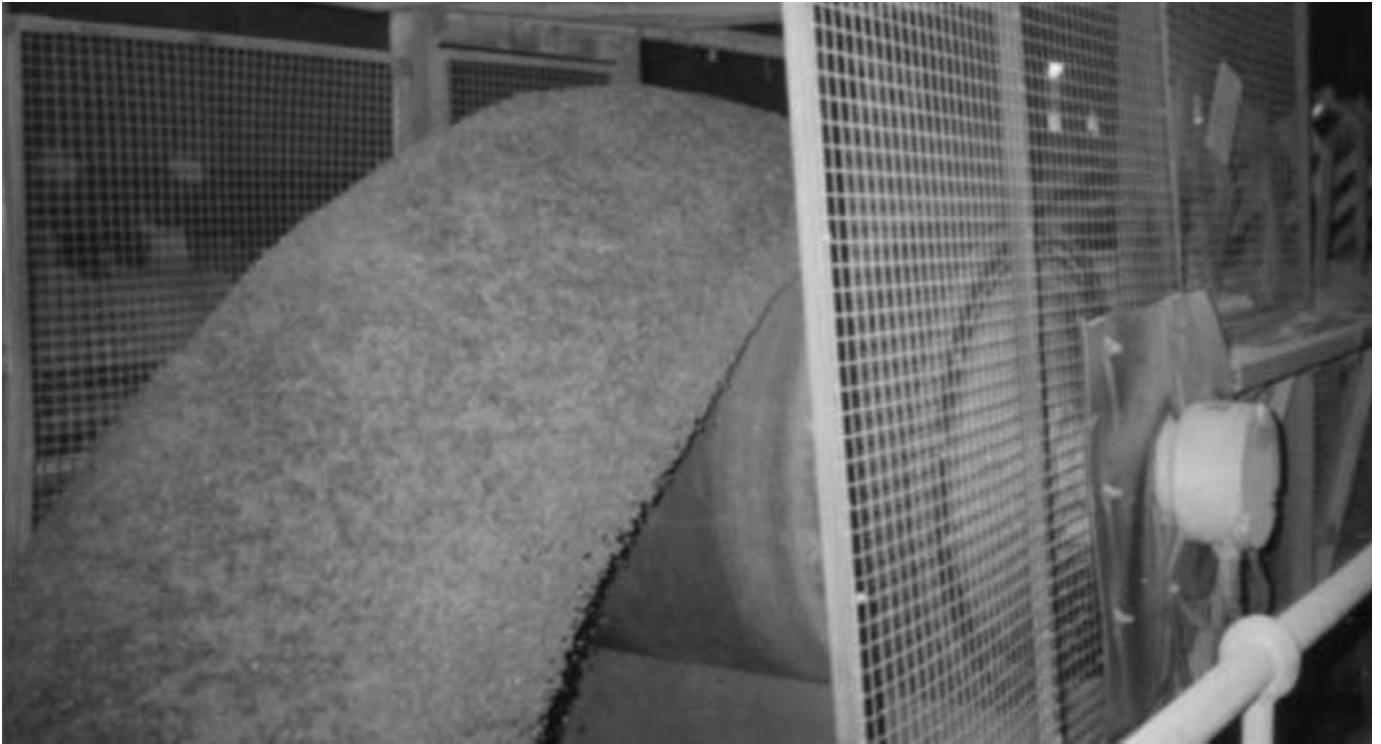
Motorized Pulleys in reversible shuttle conveyor. Application: Crushed granite. 5 Million tonnes per annum pass through this system.
