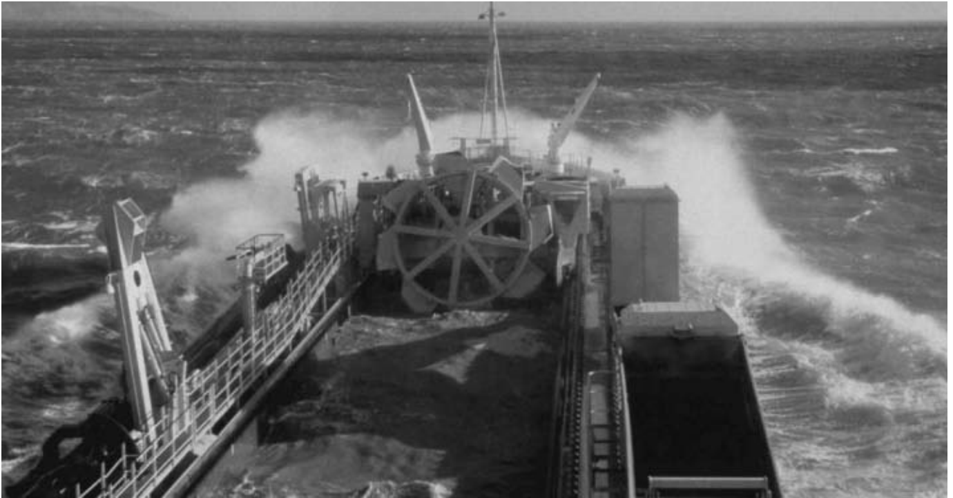
Offshore dredging in the North Sea featuring full capacity unloading at each docking to meet tide turn-round. Capacity: 2700 t/hr at up to 3.15 m/sec.
