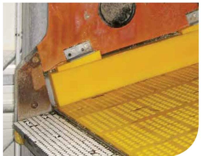
PU sideliners for flat top for CVB or TS screens
