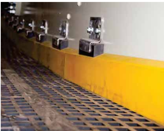
PU sideliners with chamfer top for Metso MF, mining screens
